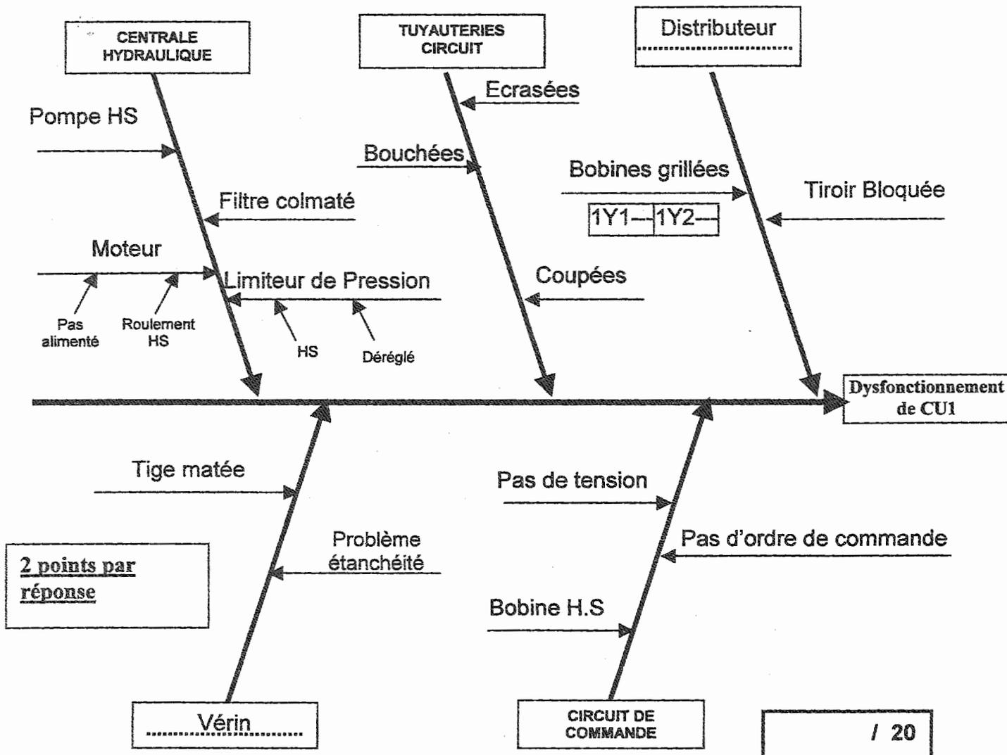
**LE CENTRE D'USINAGE CU 1 :**
