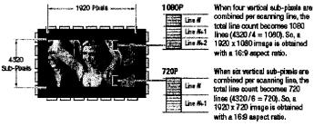
The advantage of working with this lower line count is that higher frame rates can be used for creating slo-motion effects in post production.
