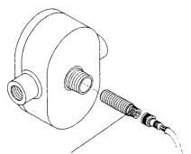
Sensor - The non-intrusive sensor threads into the side of the flowmeter. Hall Effect, Magnetic Pick-Up, high temperature, explosion-proof, and optical encoder sensors are available, in addition to a variety of flow controls and transmitters. Explosion-proof conduit connections are provided on industrial flowmeters.
