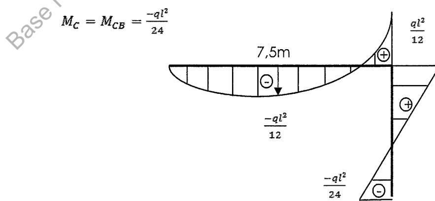
$$M_{T_{AB}} = M_{T_{0AB}} + \left( \frac{M_g + M_d}{2} \right) = \frac{-ql^2}{8} + \left( \frac{0 + \frac{ql^2}{12}}{2} \right) = \frac{-ql^2}{12}$$
