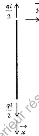
$$1.2 \quad AB : V_{(x)} = -qx + q\frac{l}{2}$$
