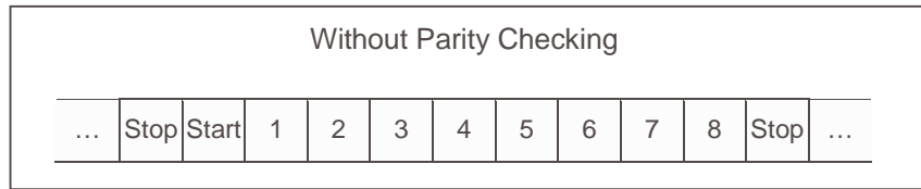
Figure 11: Bit Sequence in RTU mode (specific case of No Parity)
