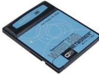
The *Spectrum24® High Rate Wireless Networker (WN)* from Symbol Technologies is a CompactFlash™ card allowing Pocket PC (Windows CE 3.0) devices to connect to a Wi-Fi™ IEEE 802.11b wireless local area network (LAN), or communicate directly with other mobile devices enabled for wireless LAN connectivity.
