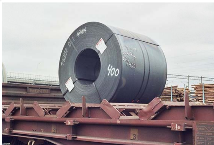
Figure 5 : Coil (bobine) en sortie du laminoir, non cisailée, non refendue
