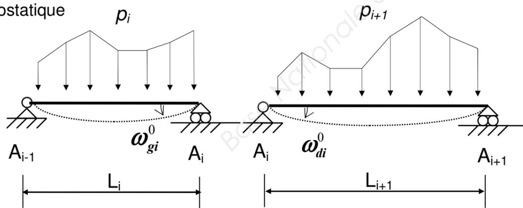
$$L_i M_{i-1} + 2(L_i + L_{i+1}) M_i + L_{i+1} M_{i+1} = 6EI(\omega_{di}^0 - \omega_{gi}^0)$$
