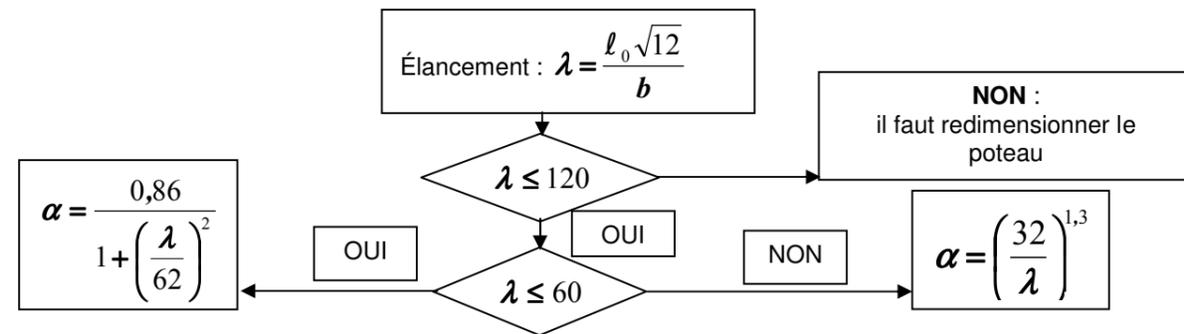
$$N_{Ed} \leq N_{Rd} \text{ et } N_{Rd} = \alpha k_h [A_c f_{cd} + A_s f_{yd}] \text{ ou } N_{Rd} = \alpha k_h A_c [f_{cd} + \rho f_{yd}]$$
