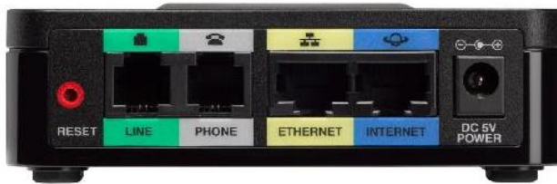
Figure 2. Ports du Cisco SPA232D
