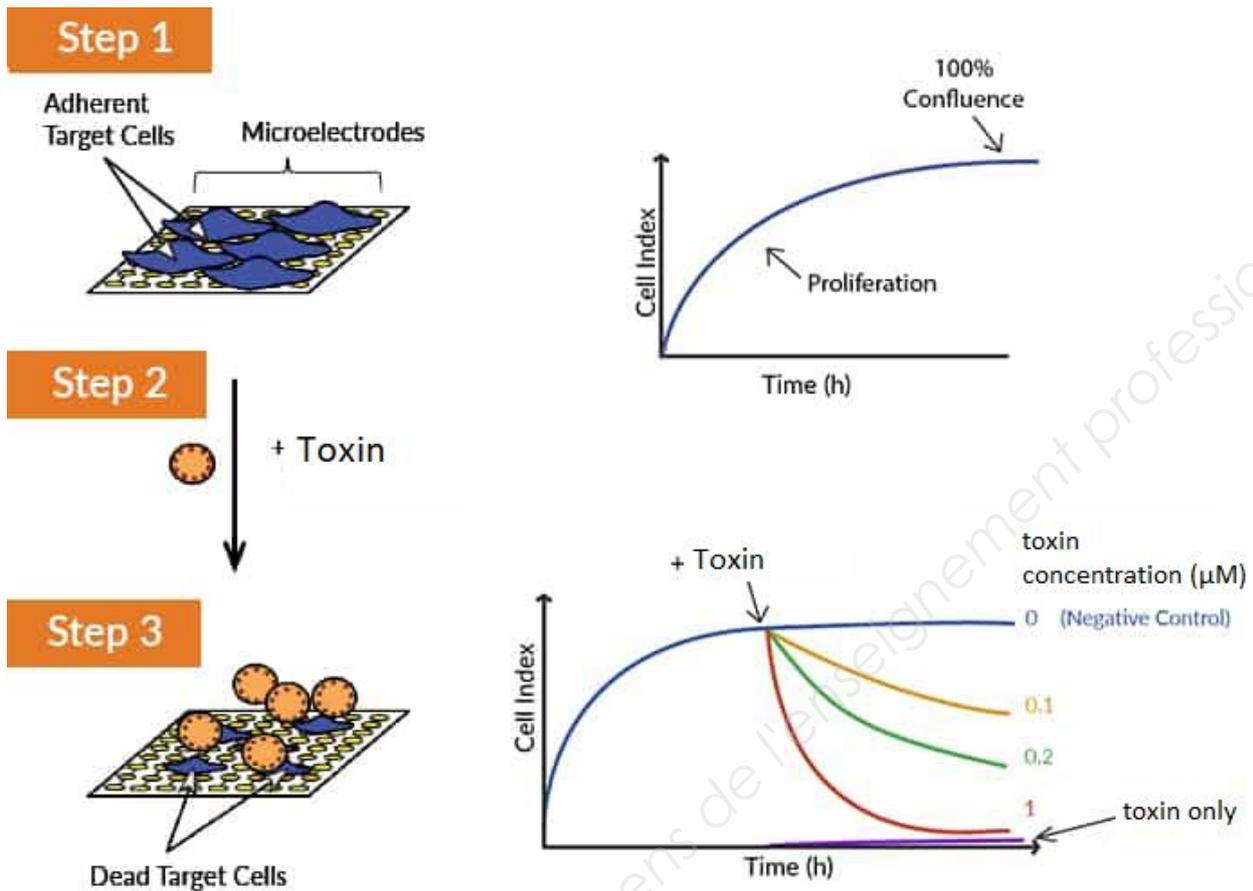
ACEA's xCELLigence® Real-Time Cell Analysis (RTCA) instruments utilize gold microelectrodes embedded in the bottom of microtiter wells to non-invasively monitor cell status including cell number, shape/size and attachment. The major distinguishing features of this technology include enhanced sensitivity, the preclusion of labels and, importantly, kinetic measurement of cell health/behavior.
