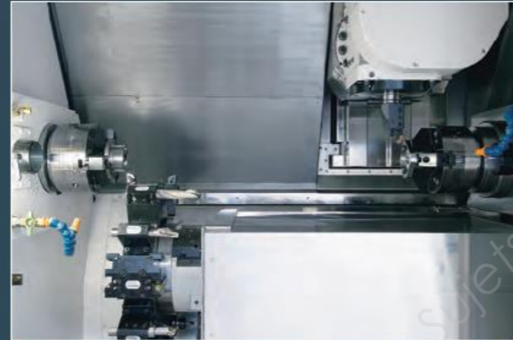
Turning / Tool spindle machining on the right hand side, lower tool on the left hand side spindle. Adjustment of the center height of cutting tool, using Y-axis positioning on upper and lower turrets, provides the possibility for high accuracy machining.
