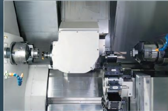
Milling on tool spindle / Drilling on lower turret With a large between spindle distance and compact tool spindle, drilling with the lower turret during machining on tool spindle can be achieved.
