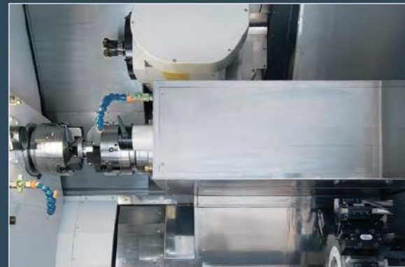
Parts transfer process By directly chucking the work piece, a highly accurate positioning and phase synchronization is obtained.
