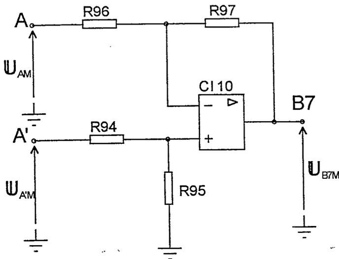
$R_{94} = R_{95} = R_{96} = R_{97} = R = 10 \text{ k}\Omega$
