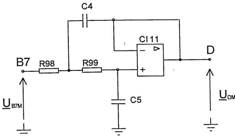
$R_{98} = R_{99} = R = 22 \text{ k}\Omega$
